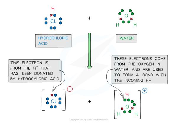
The Lewis diagram for the reaction of water with hydrochloric acid to show how water acts as a Brønsted-Lowry base and ammonia as a Brønsted-Lowry acid
