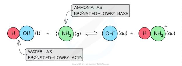
The diagram shows water acting as a Brønsted-Lowry acid by donating a proton to ammonia which accepts the proton using its lone pair of electrons
