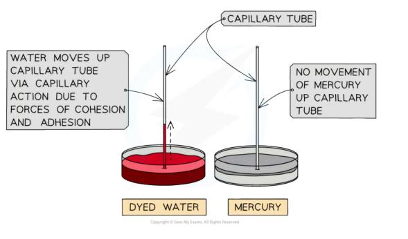
Modelling the mechanisms involved in water transport in the xylem using capillary tubing
