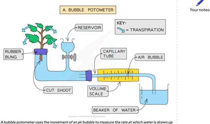
A bubble potometer uses the movement of an air bubble to measure the rate at which water is drawn up by a plant shoot. In this image the air bubble will move to the left along the tube as the plant transpires.
