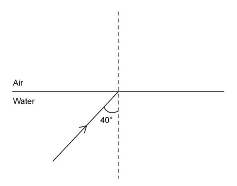
The refractive index of air is 1.00 and the refractive index of water is 1.33.
