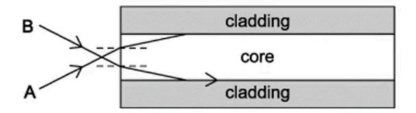
Beam A is incident at the end of the optical fibre at an angle of 12.6° to the normal and refracts into the core at 6.89° to the normal.
