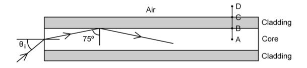
Calculate the angle of incidence  $\theta_i$  at the air–core boundary.
