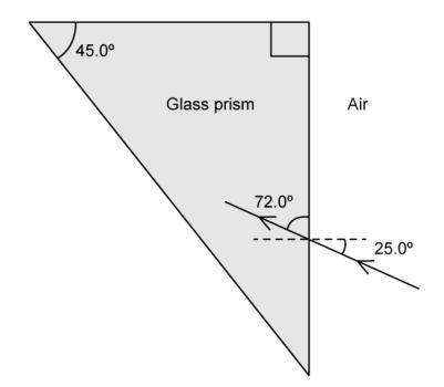
As the light ray passes through the prism, it emerges back into the air.
