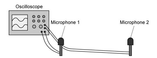
Outline how this equipment can be used to find the speed of sound.
