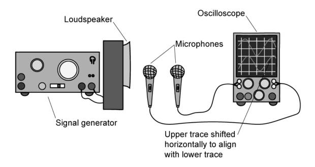
The second microphone was moved away from the first microphone until the oscilloscope traces aligned. The distance between the microphones at this point showed that the wavelength of the sound wave was 3.4 cm.
