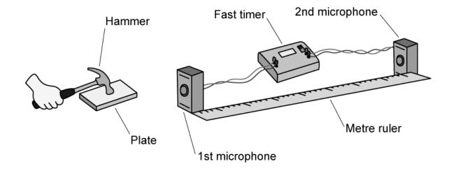
The microphones were placed 80 cm apart. The mean time interval was 2.5 ms.
