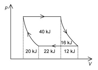
Calculate the work done by the gas during isobaric expansion.
