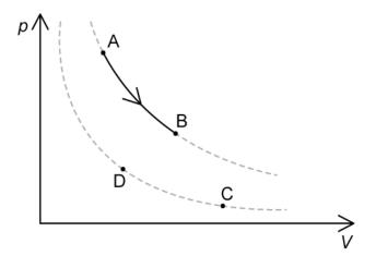
Complete the Carnot cycle by drawing the other stages on the pV diagram.
