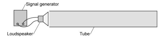
Explain how waves from the loudspeaker form stationary waves in the tube. Include in your answer a condition for formation of the wave and describe the wave which is formed.
