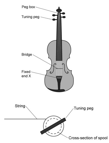
The strings are attached at end X then pass over a bridge which acts as a fixed point. The strings are also fixed at the other end, where they are wound around cylindrical spools, fixed to tuning pegs.
