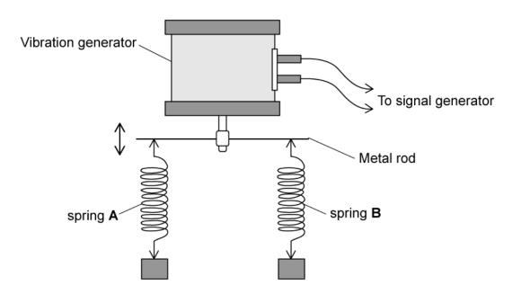
The vibration generator is connected to a signal generator. The signal generator is used to vary the frequency of vibration of the metal rod. When the signal generator is set at 6.5 Hz, the mass attached to spring A oscillates with a maximum amplitude of 4.0 cm.
