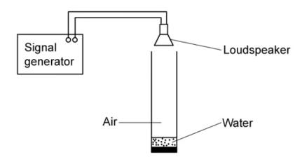
The class notice that the sound gradually increases in volume, reaching a first maximum at a particular instant. Immediately after the volume begins to decrease. Water continues to be added until the volume rises again, reaching a second and final maximum after a further  $2.5 \times 10^{-3}$  m<sup>3</sup> of water is poured in.
