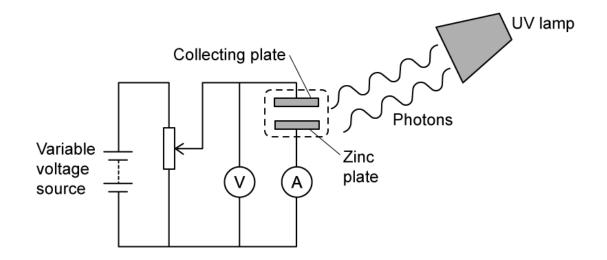
Photoelectrons are emitted from the zinc plate and move towards the positive collecting plate due to the potential difference, *V*, between the plates. When the potential difference, *V*, is varied, it is observed that the photoelectric current varies as shown on the graph.
