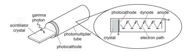
A single gamma photon incident on the scintillator crystal generates many photons of blue light. These visible light photons travel to the photocathode where they are converted into photoelectrons.
