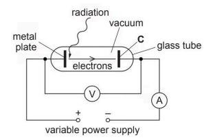
The metal plate and the electrode **C** are both in a vacuum. The electrode **C** is connected to the negative terminal of the variable power supply.
