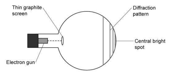
A pattern forms when diffracted electrons are incident on a fluorescent layer at the end of the tube.
