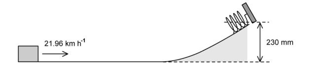
The box is momentarily brought to rest after colliding with a spring of spring constant 195 N m<sup>-1</sup>. It stops a vertical distance of 230 mm above its initial position.
