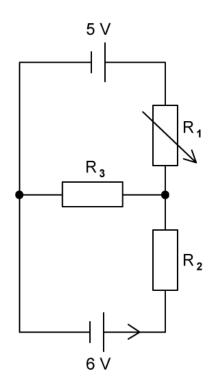
(a) Use Kirchhoff's junction law to deduce an equation for three currents  $I_1$ ,  $I_2$  and  $I_3$  at the junction between the resistors  $R_1$ ,  $R_2$  and  $R_3$ .
