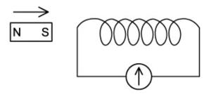
A galvanometer measures the amount of current through a moving coil, shown by a deflecting needle. A maximum deflection of the galvanometer needle of 7 units to the right is observed.
