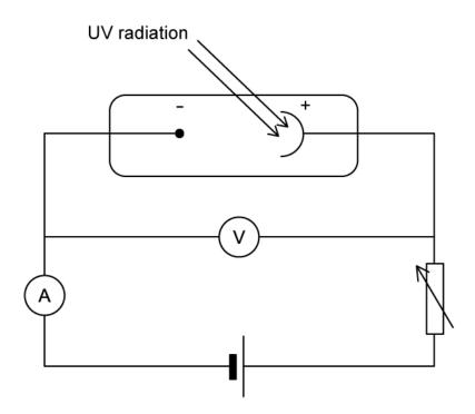
Monochromatic light of frequency *f* illuminates the cathode, which has a threshold frequency  $f_0$ . Photoelectrons are emitted and collected by the anode. A photocurrent is measured by the ammeter.
