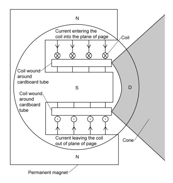
The dust cap D prevents dust from blocking the gap between the cardboard tube and the south pole of the magnet.
