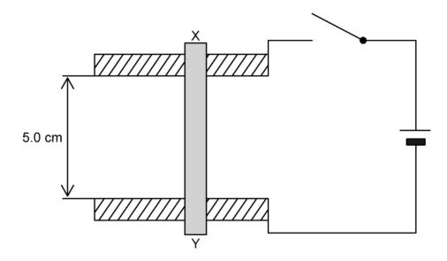
The rails can be connected to a battery to drive a current of 4.5 A through XY. A magnetic field of flux density 0.15 T acts into the screen.
