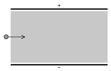
Deduce the magnetic field magnitude and direction so that an electron experiences zero net force when travelling through the plates with a speed of  $3.0 \times 10^5$  ms<sup>-1</sup>.
