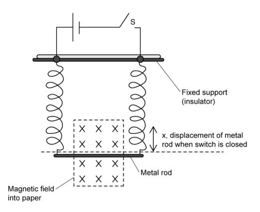
When the switch S is closed, the metal rod is displaced a distance *x* from its starting point.
