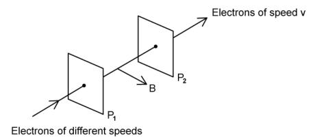
Electrons that are undeviated travel with a particular speed v along the straight line joining the holes in P<sub>1</sub> and P<sub>2</sub>.
