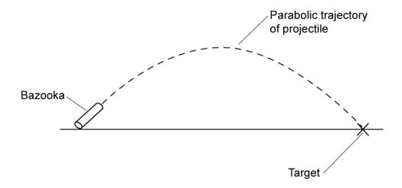
The projectile lands on its target with a final velocity *v* that can be represented as shown.
