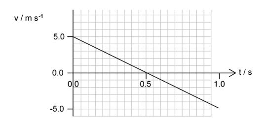
Explain why the gradient of the graph between t = 0.0 s and t = 0.5 s is roughly  $10 \text{ m s}^{-2}$ .
