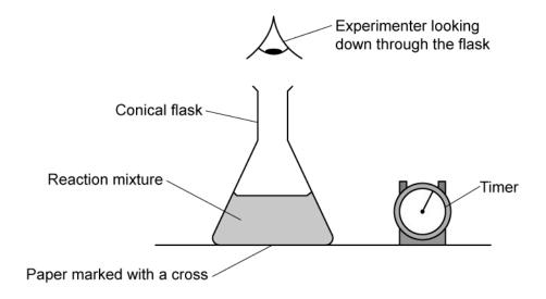
Initially they measured out 15.00 cm<sup>3</sup> of 0.900 mol dm<sup>-3</sup> hydrochloric acid and then added 40.00 cm<sup>3</sup> of 0.0150 mol dm<sup>-3</sup> aqueous sodium thiosulfate.
