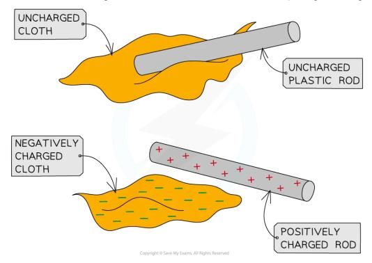
Electrons are transferred onto the cloth by friction. The cloth becomes negatively charged and the rod becomes positively charged
