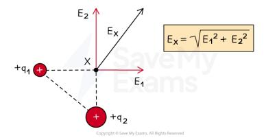
For charges which make a right-angle triangle with point X, the resultant field is the vector addition of the field due to both charges using Pythagoras theorem
