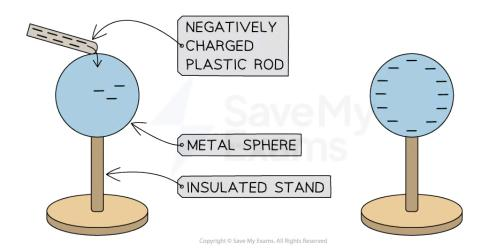
When a charged rod comes into contact with a conducting sphere, the charge flows between them
