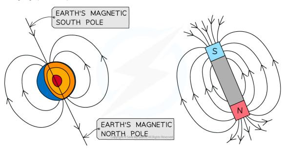
The Earth's magnetic field acts in a similar way to a bar magnet. A compass points to the Earth's magnetic south pole which is the geographic north pole
