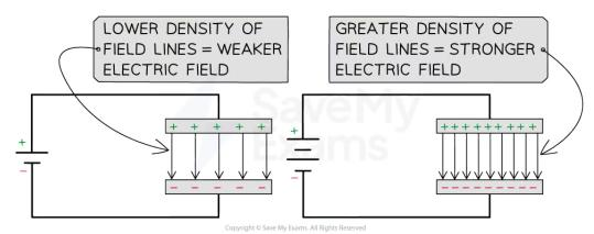
The greater the potential difference, the stronger the electric field and the greater the density of the field lines between the plates
