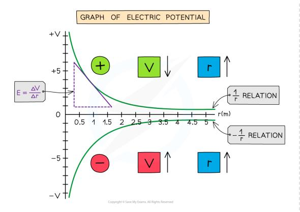
The electric potential around a positive charge decreases with distance and increases with distance around a negative charge
