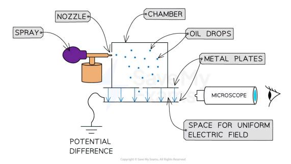
In Millikan's Oil Drop Experiment oil is sprayed into a chamber before passing between metal plates where the electric and gravitational forces are compared
