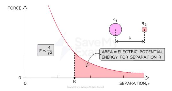
The area under the force-distance graph represents the electric potential energy of two similar point charges separated by R
