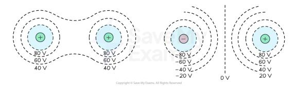
Equipotential lines show that the potential has the greatest value near the charge and decreases with distance
