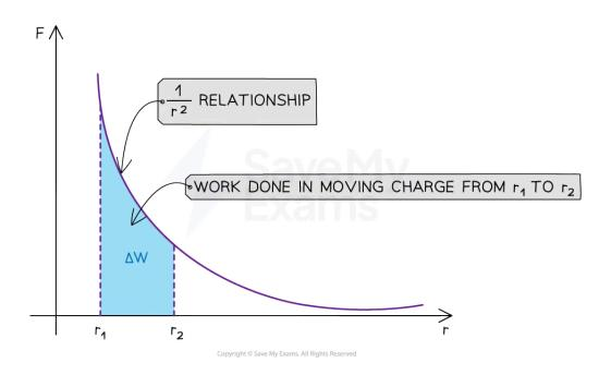
The area under a force-distance graph represents the change in electric potential energy, or the work done in moving the charge
