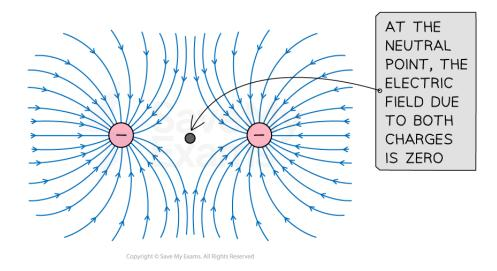
The electric field lines between two like charges are directed away from positive charges or towards negative charges. The field lines do not connect the surfaces of the charges to represent repulsion
