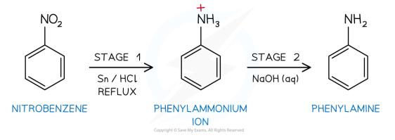
The two-stage reduction reaction of nitrobenzene to phenylamine
