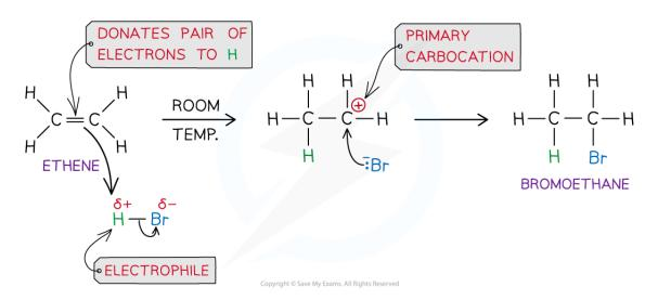
Electrophilic addition reaction of HBr and ethene to form bromoethane
