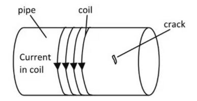
Cracks along or parallel to the length of the pipe do not show up.
