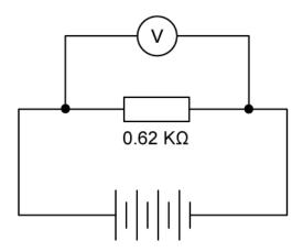
A fixed resistor with  $R = 0.62 \text{ k}\Omega$  is connected in series with the cell. A current I = 4.50 mAtravels through the circuit.
