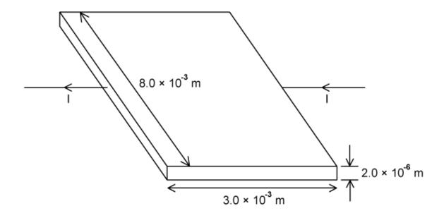
Calculate the current which passes through the carbon film when a potential difference of 2.5 mV is applied across it.
