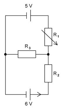
Deduce an expression for three currents  $I_1$ ,  $I_2$  and  $I_3$  at the junction between the resistors  $R_1$ ,  $R_2$  and  $R_3$ . (2 marks) (b) Initially, the variable resistor  $\boldsymbol{R}_1$  is set to 0  $\Omega$ . If  $R_2$  is 5  $\Omega$  and  $R_3$  is 10  $\Omega$ , determine the current through resistor  $R_2$ .
