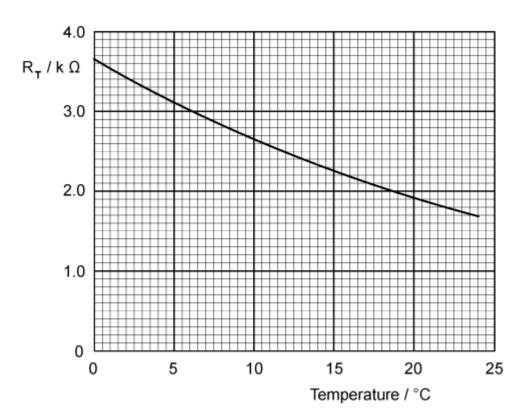
The thermistor is connected into a circuit using a power source with negligible internal resistance. The temperature is 22.5 °C.
