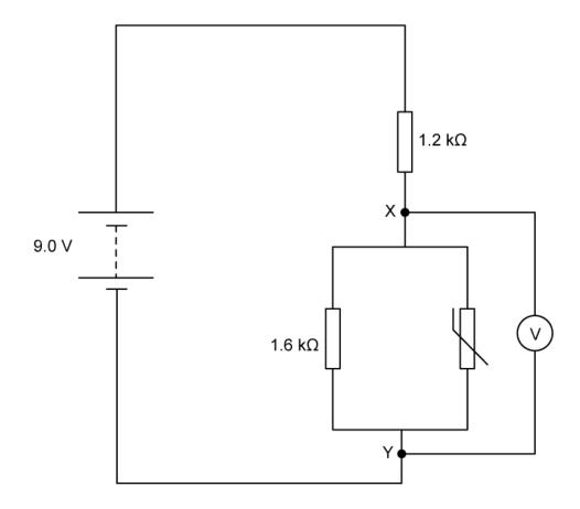
Show, without the use of a calculator, how to determine the reading on the voltmeter, giving the answer to two significant figures.
