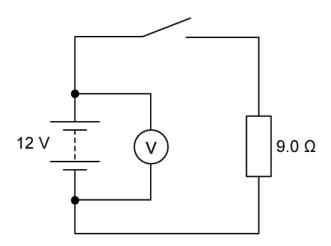
When the switch is open the voltmeter reads 12 V and when it is closed it reads 11.3 V.
