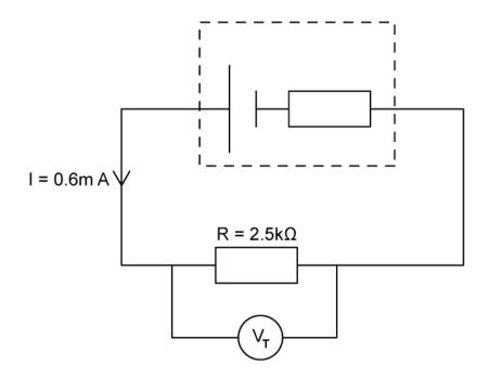
Calculate the terminal potential difference  $V_T$  of the circuit.
