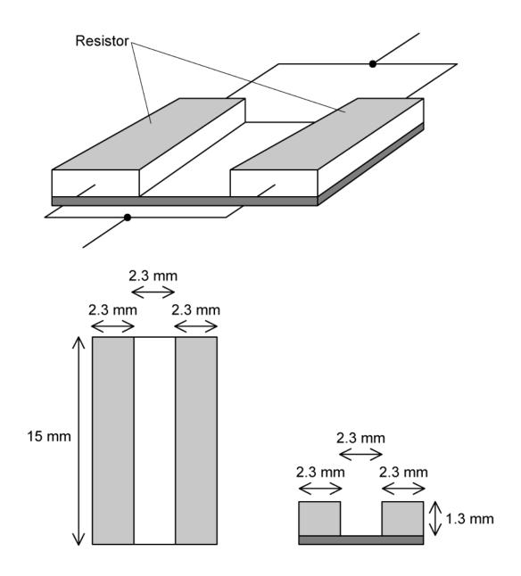
The material from which each resistor is made has a resistivity of 2.0  $\times$   $10^5\,\Omega$  m and both resistors have dimensions of 15 mm by 2.3 mm by 1.3 mm.
