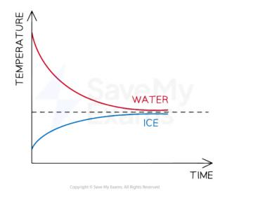
The final temperature of the water depends on the initial temperature difference between the water and ice
