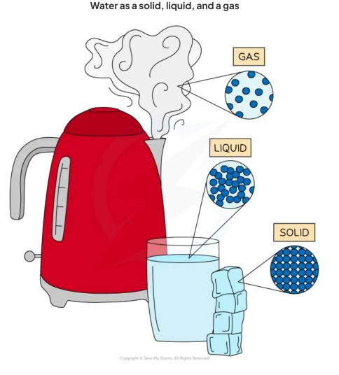
Water has three states of matter; solid ice, liquid water and gaseous steam. The difference between each state is the arrangement of the particles
