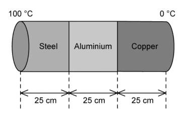
The steel end is held at 100°C and the copper end is held at 0°C.
