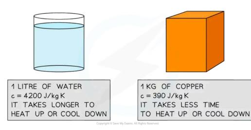
The high specific heat capacity of water means it heats up and cools down much slower than metals, such as copper
