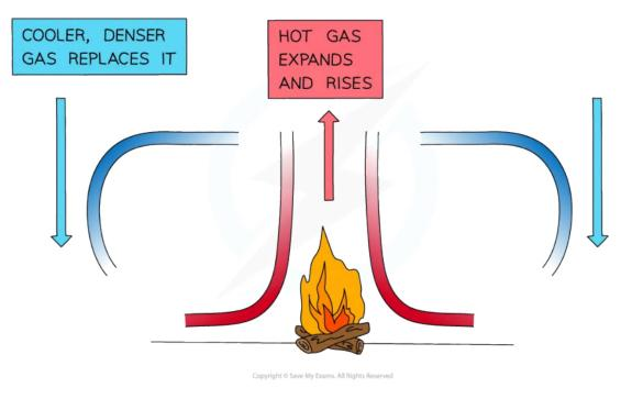
The thermal energy from a fire forms a convection current in the air around it. The hot air rises and the cool air sinks.
