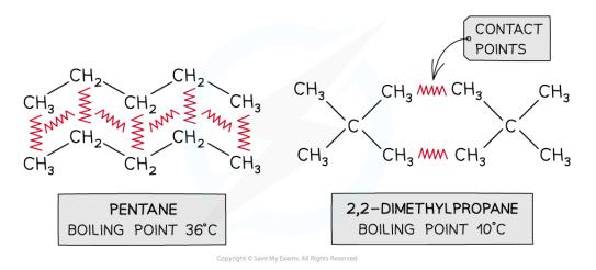
Boiling points of molecules with the same numbers of electrons but different surface areas
