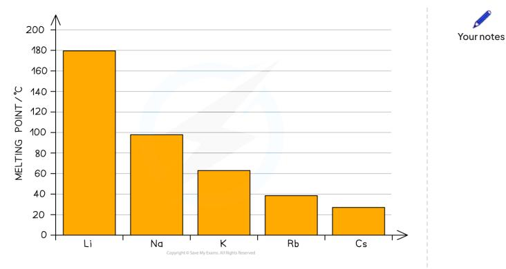
Melting points as you go down a group of metals. The metallic bonding gets weaker from Li to Cs
