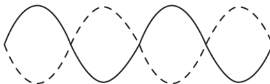
Standing waves produced at varying frequencies
