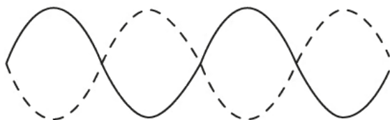
Standing waves produced at varying frequencies
