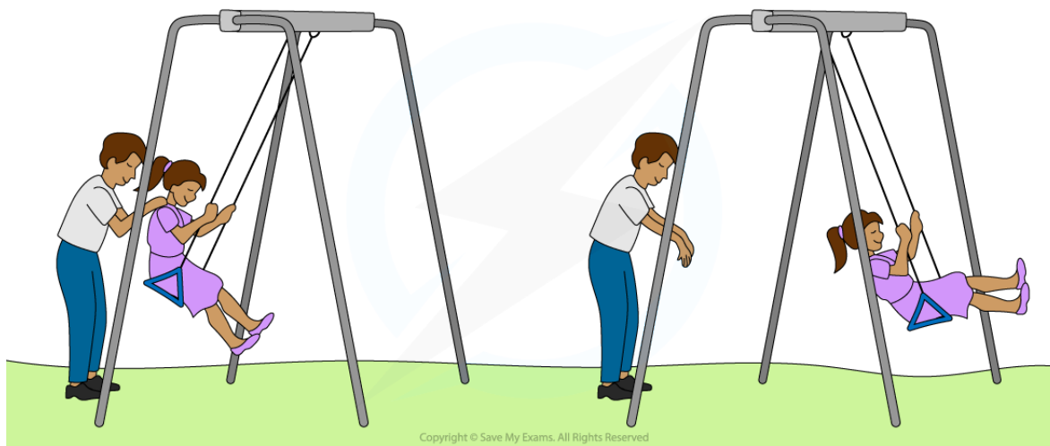
Pushing a child on a swing is an example of how forced oscillations can produce resonance
