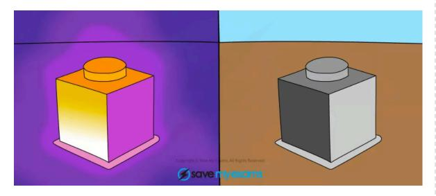
An image of a hot object, known as a Leslie cube, taken in both Infrared and visible light. The black surface emits more thermal radiation (infrared) than the shiny surface
