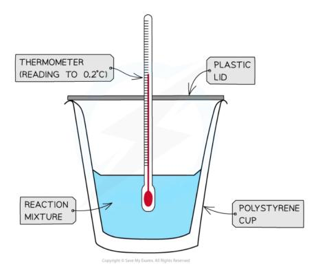
A polystyrene cup can act as a calorimeter to find enthalpy changes in a chemical reaction
