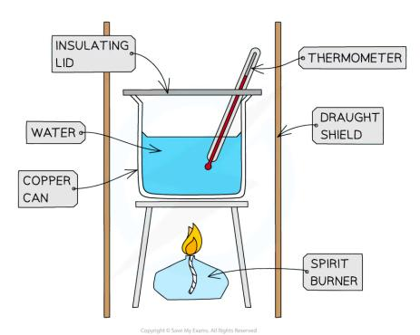
You should be able to state what the impact would be of not using a draught shield in a simple combustion calorimetry experiment
