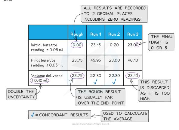
Calculating the average volume delivered in a titration should not include non-concordant volumes.
