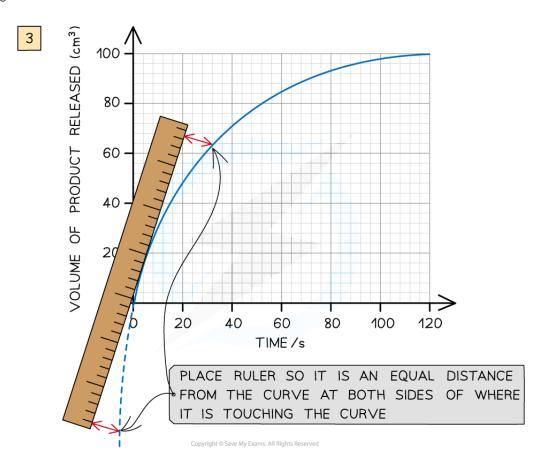
Lining up a ruler against the curve is essential to drawing a tangent accurately
