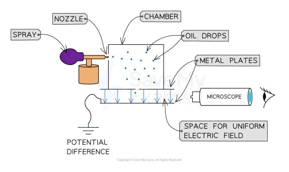
In Millikan's Oil Drop Experiment oil is sprayed into a chamber before passing between metal plates where the electric and gravitational forces are compared
