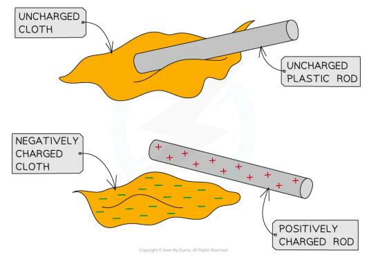
Electrons are transferred onto the cloth by friction. The cloth becomes negatively charged and the rod becomes positively charged
