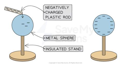
When a charged rod comes into contact with a conducting sphere, the charge flows between them
