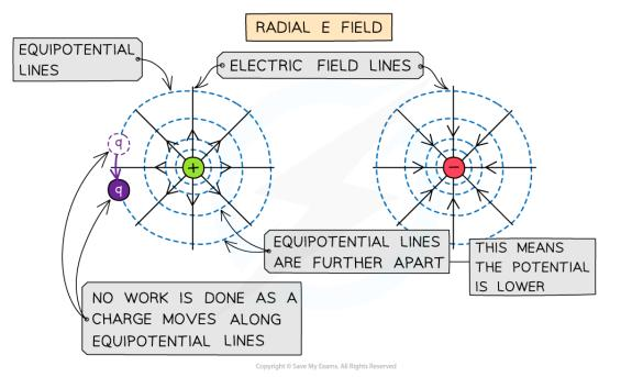
Equipotential lines for a radial electric field are concentric circles which increase in radius and are perpendicular to the field lines
