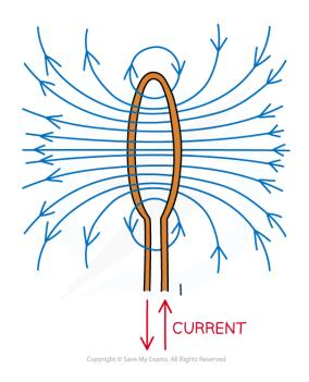
Magnetic field lines of many individual circular coils can be combined to make a solenoid
