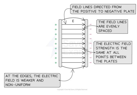
Electric field lines between two parallel plates are directed from the positive to the negative plate. A uniform electric field has equally spaced field lines
