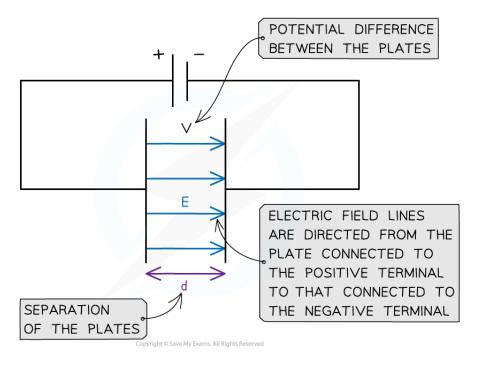
The electric field strength between two charged parallel plates is the ratio of the potential difference and separation of the plates
