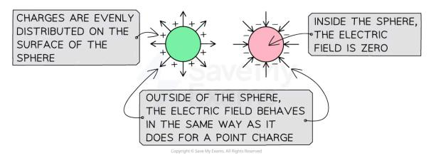
Electric field lines around a charged conducting sphere are similar to the field lines around a point charge
