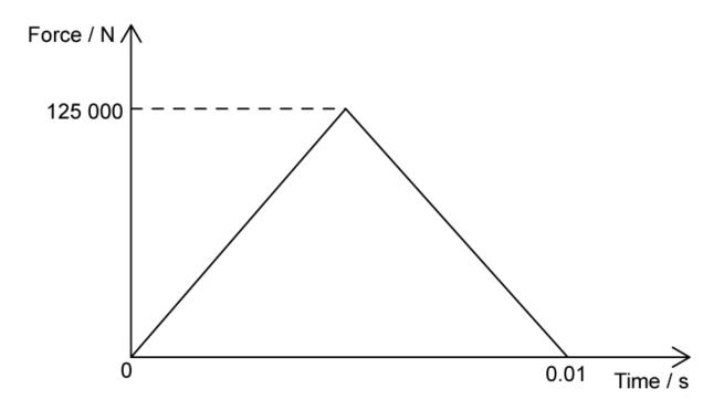
Use the graph to show that the impulse of the collision is 625 Ns.
