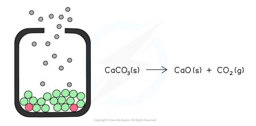
The diagram shows an open system in which the calcium carbonate is continually decomposing as the carbon dioxide is lost causing the reaction to eventually go to completion
