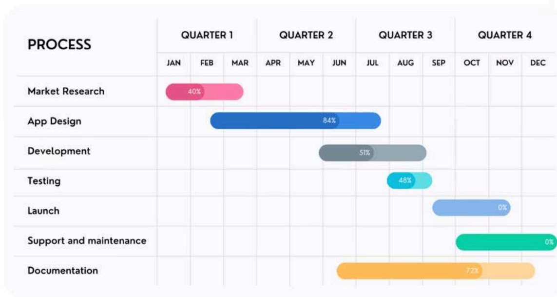
An example of a simple Gantt chart used to plan the development and launch of a web app
