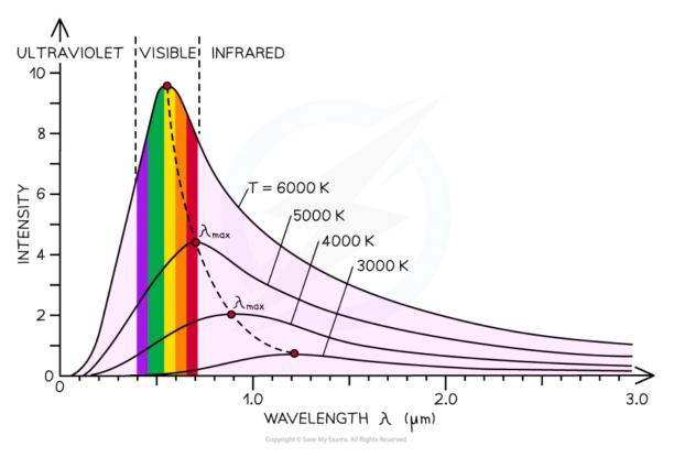
The intensity-wavelength graph shows how thermodynamic temperature links to the peak wavelength for four different bodies
