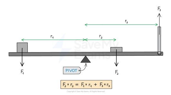
When the resultant force and resultant torque are both zero, the beam will be in rotational equilibrium
