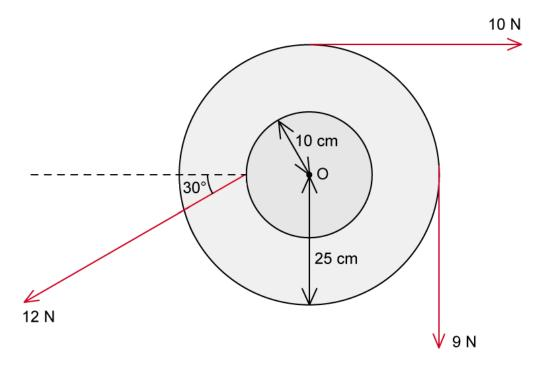
Determine the net resultant torque about the axis of rotation O. State whether the angular acceleration that is produced is clockwise or anticlockwise.
