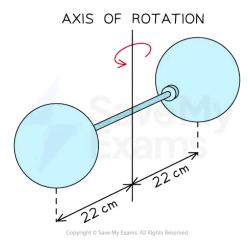
Moment of inertia of a thin rod about its centre =  $\frac{1}{12} mL^2$
