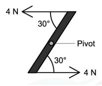
Determine the magnitude of the torque of the couple on the ruler.
