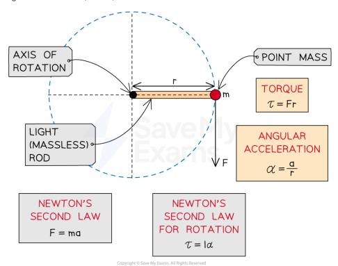
Newton's second law for rotating bodies is equivalent to Newton's second law for linear motion
