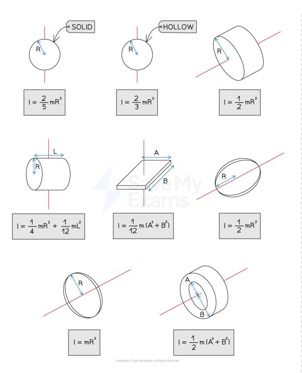
Moments of inertia of common shapes, where R represents radius and L represents length, as shown
