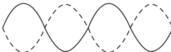
Standing waves produced at varying frequencies
