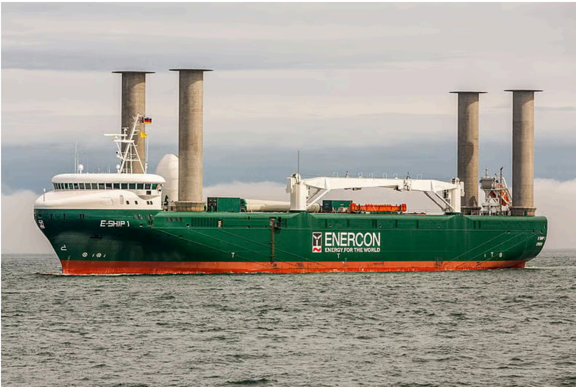
Cargo ship with four large rotor sails (photo by Alan Jamieson, from Wikimedia Commons)
