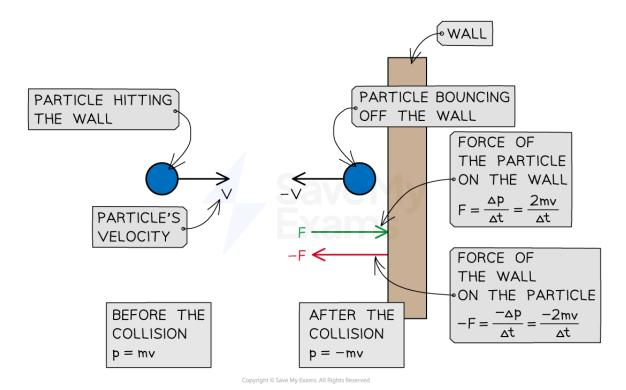
A particle hitting a wall of the container in which the gas is held experiences a force from the wall and a change in momentum. The particle exerts an equal and opposite force on the wall
