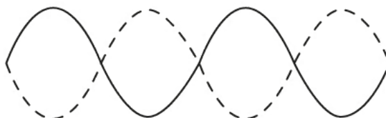
Standing waves produced at varying frequencies
