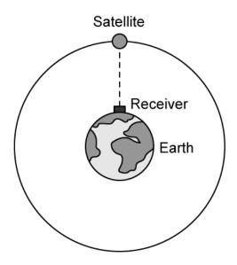
When the satellite is directly overhead the microwave signal reaches the receiver 62 ms after leaving the satellite.
