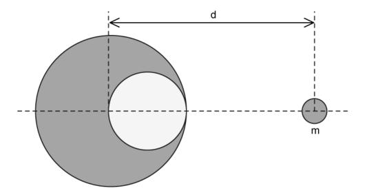
Show that the magnitude of the force *F* exerted by the spherical hollow on a small mass *m*, placed at a distance *d* from its centre, is given by:
