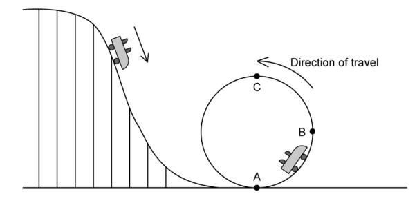
As the passengers move around the circle from **A** to **B** to **C**, the reaction force between exerted by their seat varies.
