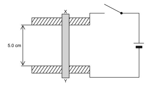
The rails are connected via a switch to a cell that can drive a current of 4.5 A through XY. A magnetic field of flux density 0.20 T acts into the screen.
