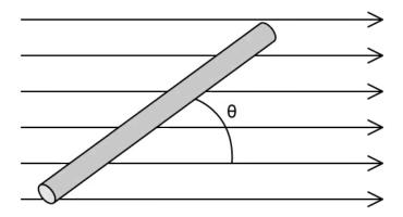
The force acting on the current-carrying conductor when it lies at different angles to the field can be calculated using the equation
