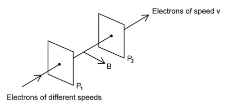
Electrons that are undeviated travel with a particular speed v along the straight line joining the holes in  $P_1$  and  $P_2$ .
