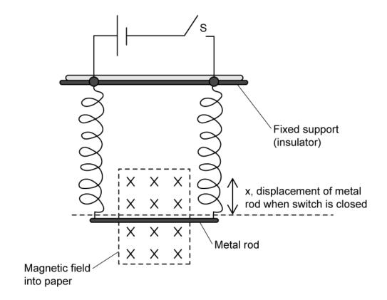
When the switch S is closed, the metal rod is displaced a distance x from its starting point.
