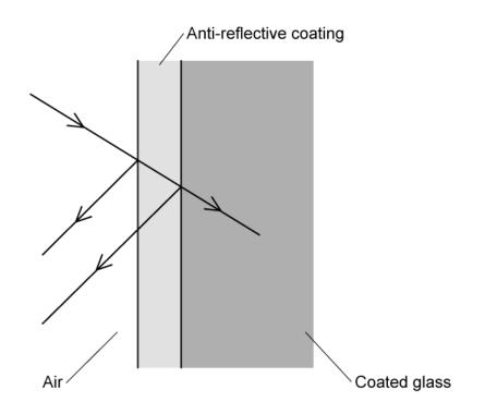
The coating is designed such that there is a phase shift of  $\pi$  radians at the first boundary (between the air and the coating) as well as at the second boundary (between the coating and the glass).
