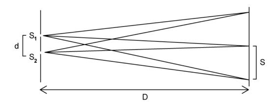
The distance between the bright fringes depends on the wavelength of the incident light.
