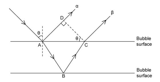
Upon reflection, ray lpha undergoes a phase shift of  $\pi$  radians. Ray eta does not undergo any phase shift upon reflection.
