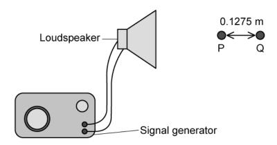
Determine the wavelength,  $\lambda$ , of the sound wave.
