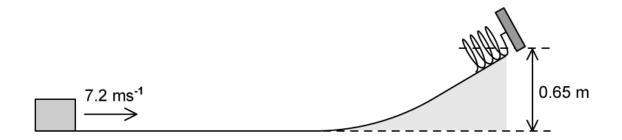
The box is momentarily brought to rest after colliding with a spring of spring constant  $210 \text{ N m}^{-1}$ . It stops a vertical distance of 0.65 m above its initial position.
