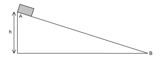
The object is released and slides down the slope from A to B with negligible friction. Assume that the potential energy is zero at B.
