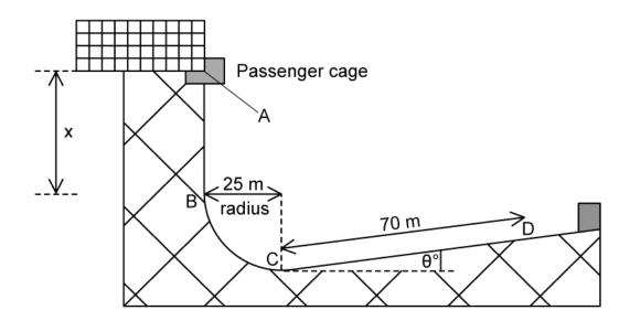
The total mass of the cage and passengers is  $3.556 \times 10^2$  kg. The average resistive force exerted by the brakes between C and D is  $4.4 \times 10^3$  N.
