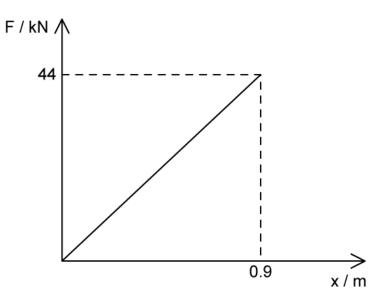
Using the area under the graph, show that the spring constant of the spring is about 49 kN  $m^{-1}$ .
