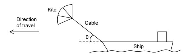
The tension in the cable that connects the kite to the ship is 475 kN. The kite is pulling on the ship at an angle of  $\theta$  to the horizontal plane of the ship's deck. The ship travels at a steady speed of 14.76 km hr<sup>-1</sup> when its engines operate with a power output of 5.9 MW. The work done by the engines is 0.365 GJ when turned on for 0.09 hours.
