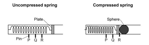
A student hypothesises that the spring constant of the spring inside the launcher has the same value for different compression distances.
