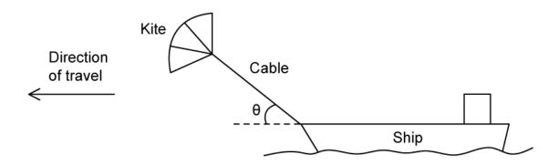
The tension in the cable that connects the kite to the ship is 350 kN. The kite is pulling the ship at an angle of  $\theta$  to the horizontal. The ship travels at a steady speed of 3.9 m s<sup>-1</sup> when the ship's engines operate with a power output of 5.7 MW.
