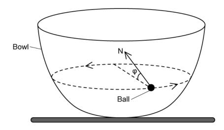
The normal reaction force N makes an angle  $\phi$  to the plane of the ball's path. Ignore the effects of friction.
