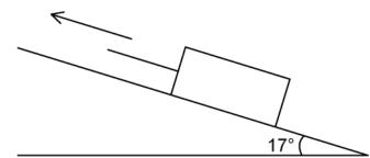
The incline makes an angle of 17° with the horizontal. The mass of the block is 180 kg and the tension *T* in the cable of 0.9 kN.
