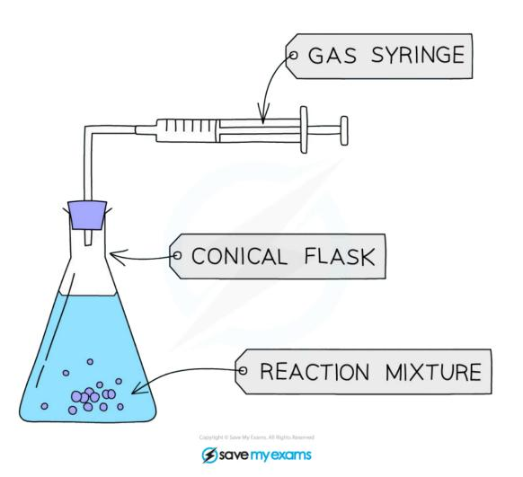
Gas syringes can be used to measure the volume of gas produced in a reaction
