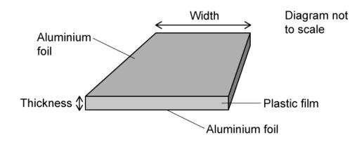
The aluminium foil has an area of 0.28  $m^2$  and the plastic film has a permittivity of 2.5  $\times$  10^{-11} C^2 N^{-1} m^{-2}.
