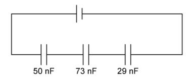
Calculate the combined capacitance in this circuit.
