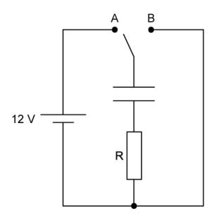
Initially, the vacuum capacitor is uncharged. At a time of t = 0 s, the switch is placed at position A. The voltage across the capacitor is recorded over time and plotted in the graph below.
