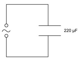
The power supply is adjusted such that the initial voltage is 6.0 V and the alternating voltage frequency is 4000 rad s<sup>-1</sup>.
