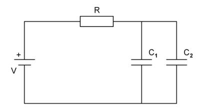
State the effect on the charge stored in the circuit after adding this additional capacitor.
