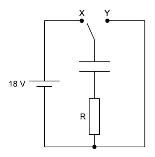
At t = 0 the switch is placed at position Y. The graph shows the variation with time t of the voltage V across the capacitor. The capacitor has capacitance 2.8  $\mu$ F in a vacuum.
