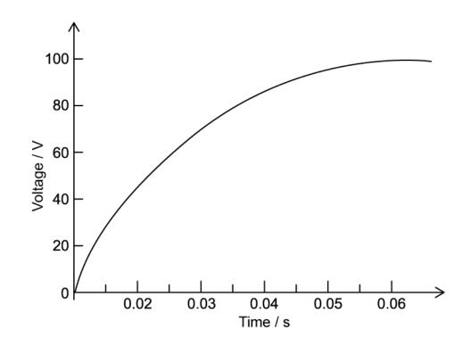
Use the graph to state the value of the time constant for this new circuit.
