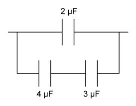
Calculate the combined capacitance of the capacitors.
