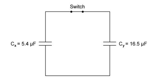
Use this value to calculate the magnitudes of both charges,  $q_X$  and  $q_Y$  after the switch has closed and charge has stopped moving.
