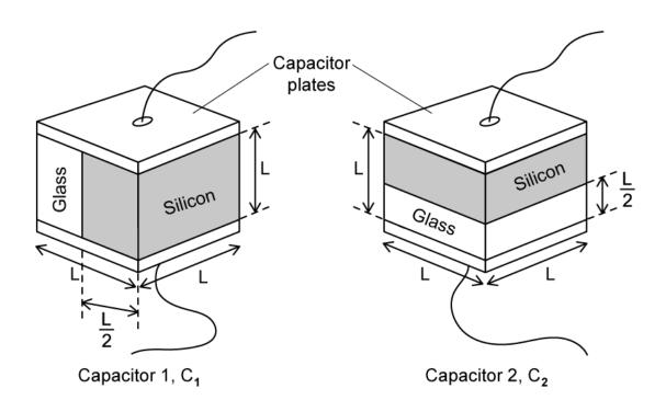
The capacitor with the dielectric split vertically has a capacitance of  $C_1$  and the capacitor with the dielectric split down the middle has a capacitance of  $C_2$ .
