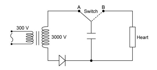
Calculate the maximum energy stored in the capacitor.
