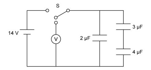
The switch is first connected to the d.c. supply.
