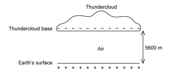
The lower plate of the capacitor is the Earth's surface and the upper plate is the base of the thundercloud.
