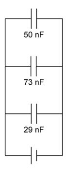
Determine the new total capacitance of the circuit.
