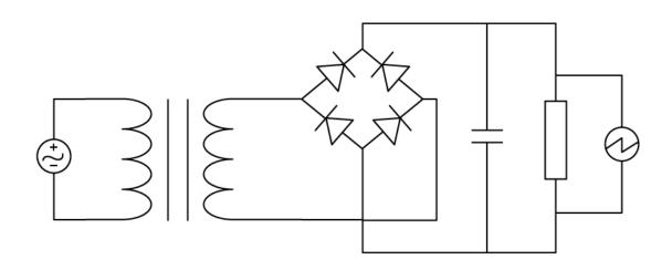
Sketch the expected graph of the output voltage for this circuit.
