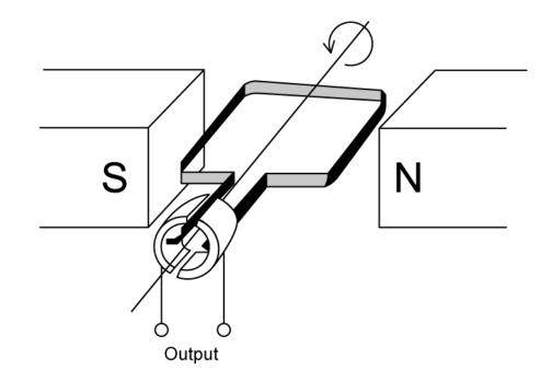
The power output varies over time for a generator rotating with a maximum power output of  $P_0$  and a frequency of 20 Hz.
