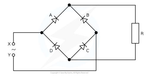
Identify which diodes are conducting when terminal X of the ac generator is negative.
