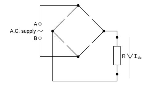
Complete the sketch to show an arrangement of diodes which would achieve full rectification with dc current in the load in the direction shown.
