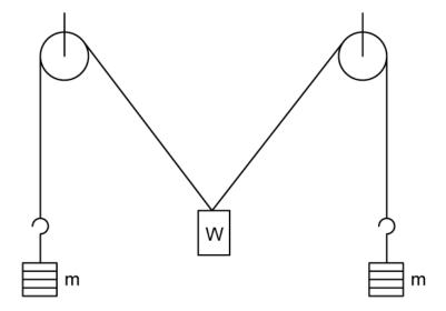
Draw a free body force diagram for the load W, expressing tensional forces in terms of each mass *m*.
