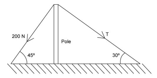
Construct a scale diagram to determine the weight of the pole W and the magnitude of Т.
