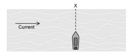
Draw a vector triangle to show the velocities of the motorboat in still water, the current and the resultant velocity of the motorboat.
