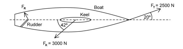
By calculation, or by constructing a diagram, determine the magnitude of  $F_{\rm R}$ .
