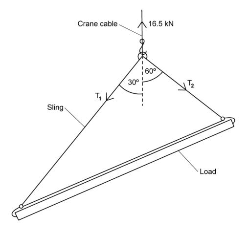
Construct a diagram, including an appropriate scale, to determine the magnitude of  $T_1$ and  $T_2$ . (4 marks) (d) A crate rests on an inclined plane.
