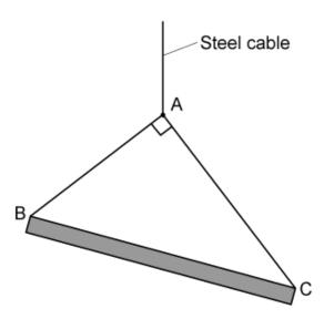
Draw the vector triangle for this situation labelling the tension in both cables and the weight of the beam.
