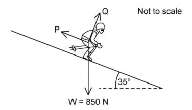
The force labelled  ${\bf P}$  is parallel to the slope. The force labelled  ${\bf Q}$  is perpendicular to the slope. Assume that there is no friction between the skis and the snow.
