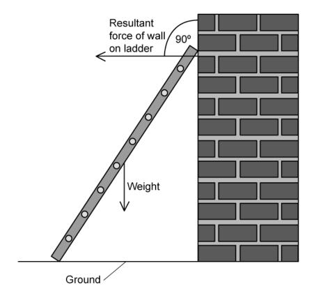
Explain how the image shows that there is no coefficient of static friction between the ladder and the wall.
