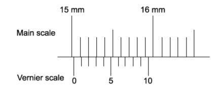
Determine the full reading of the vernier calliper with its absolute uncertainty.
