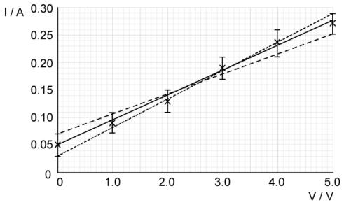
Black solid line = best fit line Dashed black line = maximum fit line Dotted black line = minimum fit line
