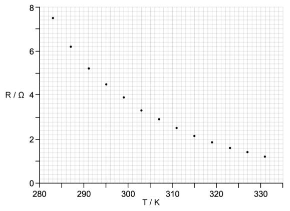
The electric current through the thermistor for T = 283 K is 0.0078 mA.
